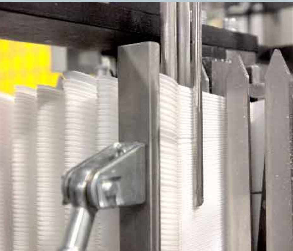
Eight frames of 18 spoons will make up a larger frame of 144 spoons, above. The larger frames are stacked to a height of 125 frames, below left, and packaged, below right.
