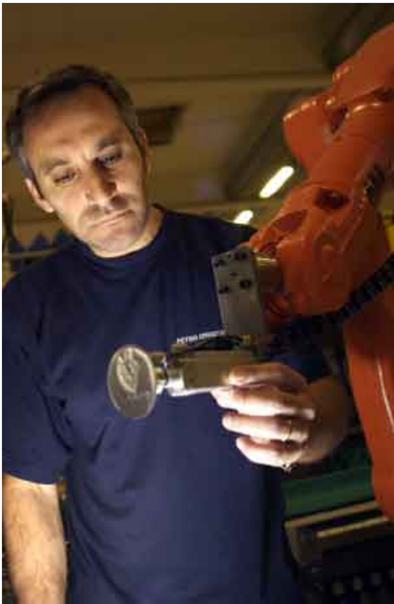
Operator Aziz Dal checks the vacuum grip of the IRB 1600 robot on a car emblem.
