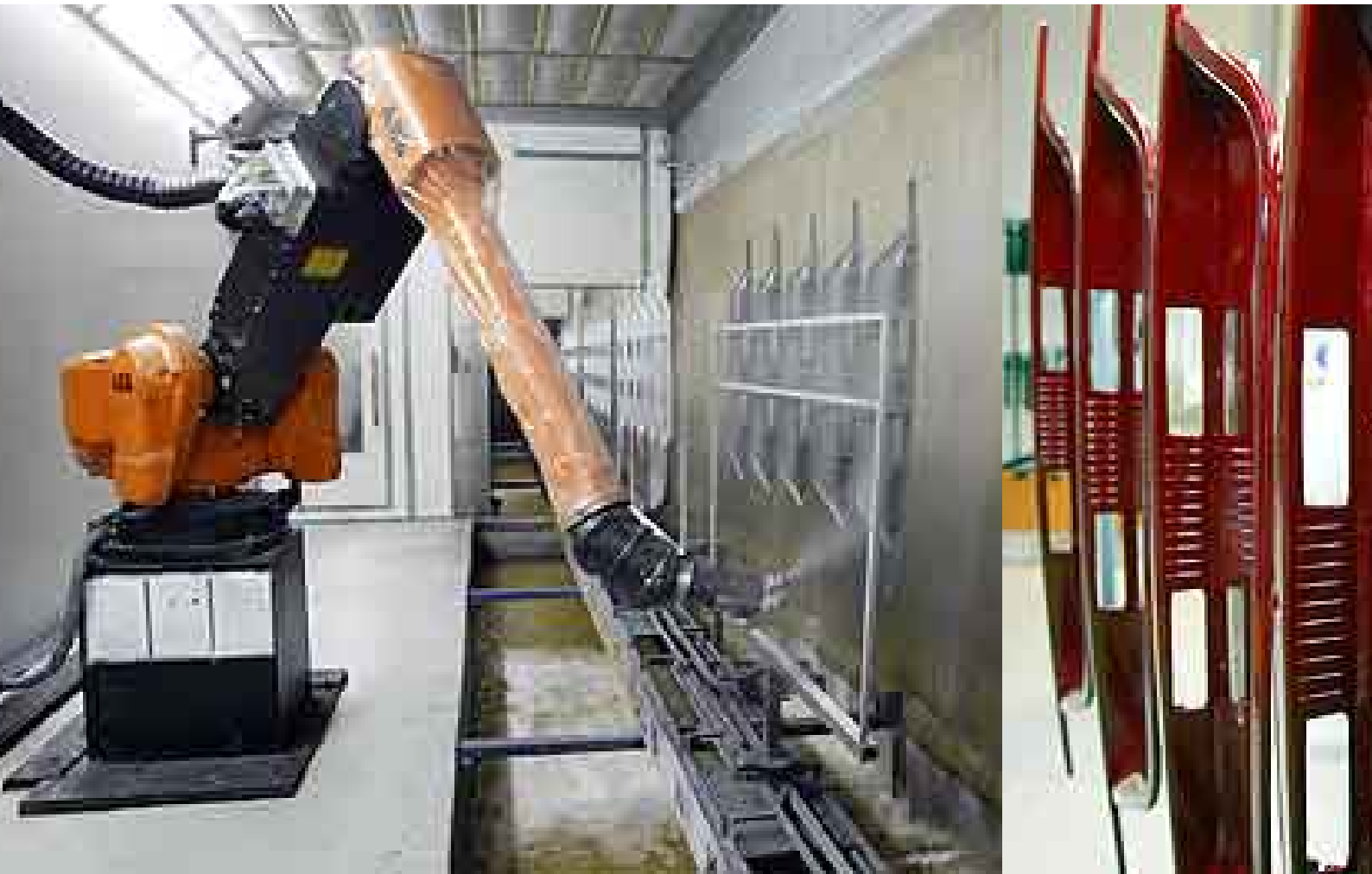
An IRB 5400 robot spraypaints the backs of rear parcel shelf brake light housings at D&M.
