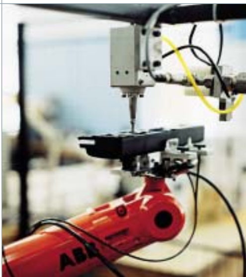
An ABB IRB 1400 robot assembles a boat trim board before it undergoes heating.
