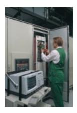
The ABB ACS 600 Modules and Rittal TS cabinets were assembled for testing in ABB's Lampertheim factory, Germany. Some mechanical parts were also designed and tested to make it easier to use the ACS 600 product combinations. Several strict performance tests were made on the combinations in ABB's Helsinki factory. In particular, the cooling of the cabinet was thoroughly tested and measured.
