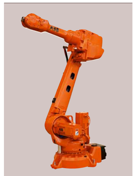
The IRB 2600-20/1.85 with an increased arm reach of 1.85 m (instead of 1.65)
