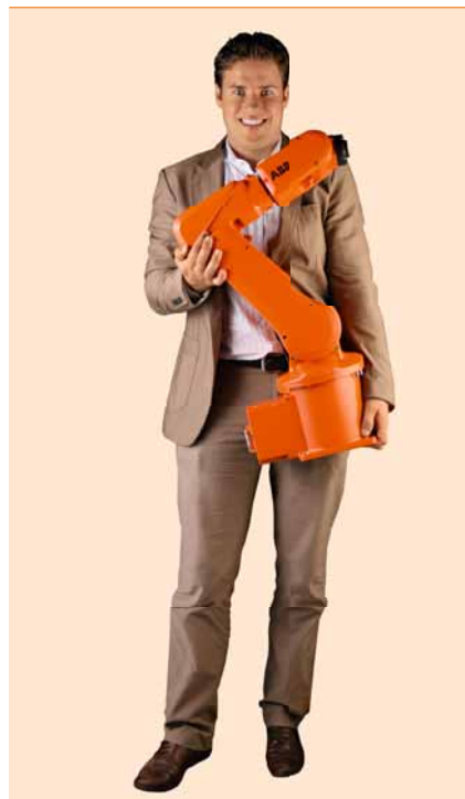
2 The IRB 120 weighs in at 25 kg
