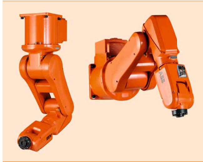
1 The IRB 120 can be mounted in a wide range of positions. Here, it is mounted from the ceiling (left) and a wall (right).
