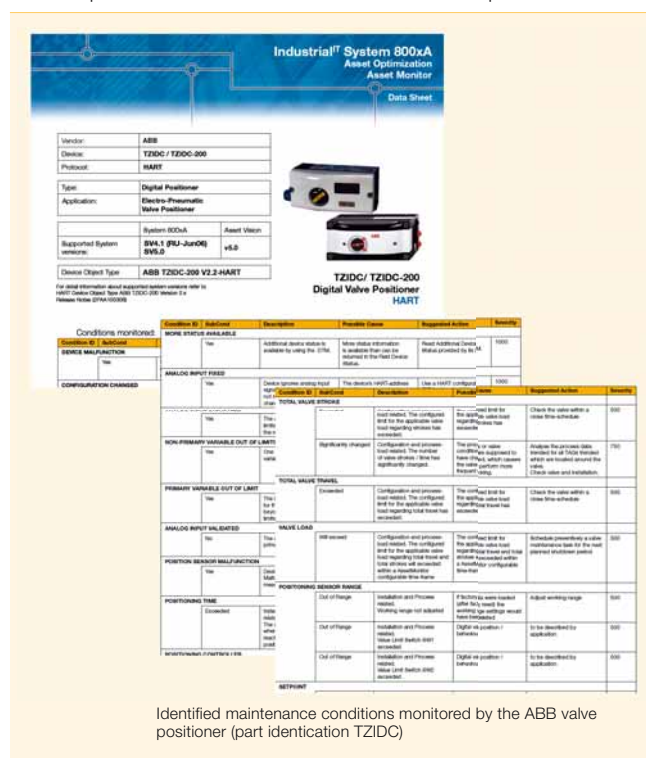
2 Example of detectable conditions for control valve positioner
