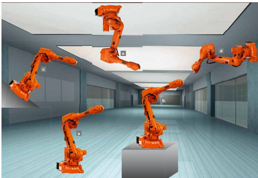
3 Mounting variants of the IRB 2600: floor a , shelf b , tilted c , wall d and inverted e
