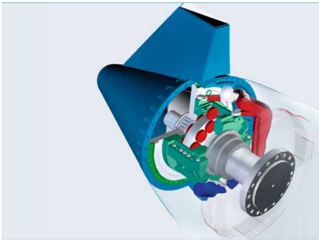
3 Model of the new hybrid bearing developed for the Azipod XO
