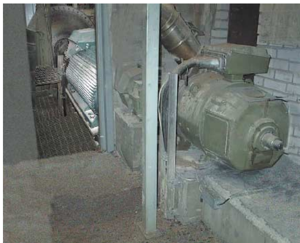
Fig 1. Metsä-Serla, Kirkniemi Direct Drive running in a PM1 dryer section since July 1999, replaced old DC motor and gear in front.
