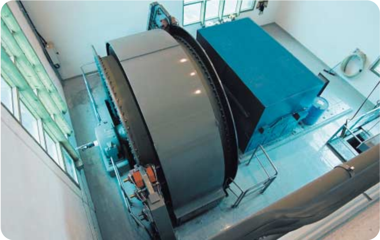
Fig. 4. 4.5 diameter friction hoist with synchronous motor drive.
