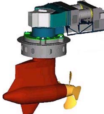
Azipod marine propulsion
