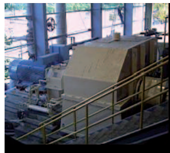
View of the cane mill (862 kW) and ACS 1000 controlling the cane mill at Santa Matilde mill of Compania Azucarera Hondurena S.A..
