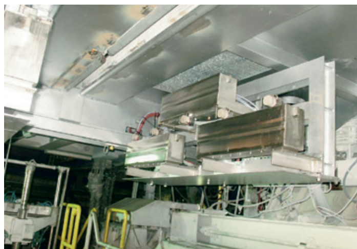
The EM Stabilizer module installed under the hot gauge platform.
