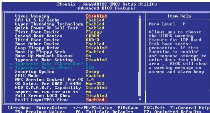
The screen above list all the fields available in the Advanced BIOS Features submenu, for ease of reference in this manual. In the actual CMOS setup, you have to use the scroll bar to view the fields. The settings on the screen are for reference only. Your version may not be identical to this one.
