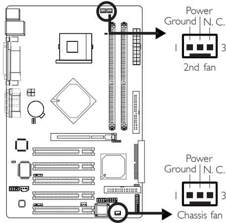
The chassis fan connector (J11) and 2nd fan connector (J10) are used to connect cooling fans. The cooling fans will provide adequate airflow throughout the chassis to prevent overheating the CPU and system board components.
