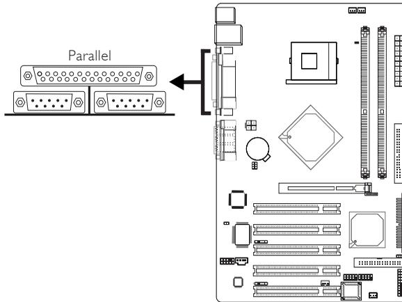
The system board has a standard parallel port (Burgundy) at location CN8 for interfacing your PC to a parallel printer. It supports SPP, ECP, EPP and PntMode.
