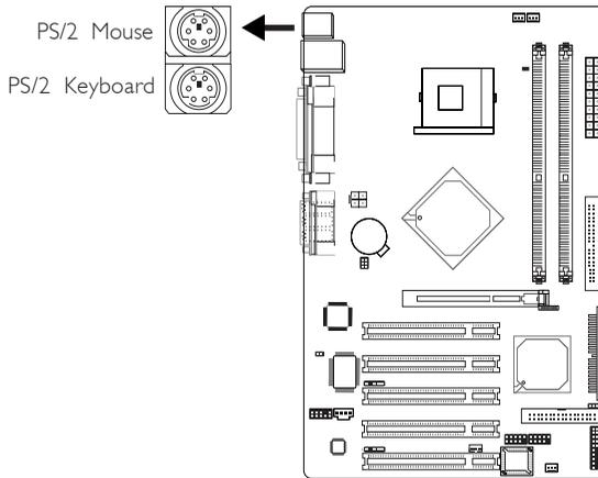
The system board is equipped with an onboard PS/2 mouse (Green) and PS/2 keyboard (Purple) ports - both at location CN1 of the system board. The PS/2 mouse port uses IRQ12. If a mouse is not connected to this port, the system will reserve IRQ12 for other expansion cards.
