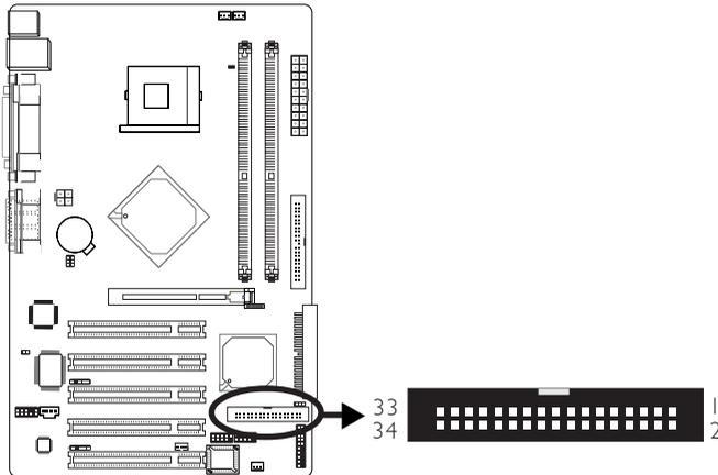
The system board is equipped with a shrouded floppy disk drive connector that supports two standard floppy disk drives. To prevent improper floppy cable installation, the shrouded floppy disk header has a keying mechanism. The 34-pin connector on the floppy cable can be placed into the header only if pin 1 of the connector is aligned with pin 1 of the header.
