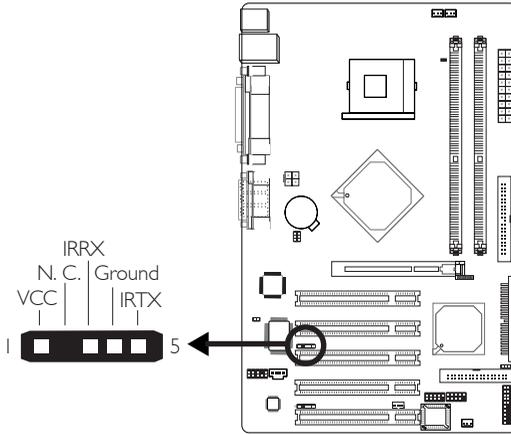
Connect your IrDA cable to connector J5 on the system board.
