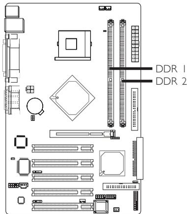
The system board supports DDR SDRAM DIMM. Double Data Rate SDRAM (DDR SDRAM) is a type of SDRAM that doubles the data rate through reading and writing at both the rising and falling edge of each clock. This effectively doubles the speed of operation therefore doubling the speed of data transfer.
