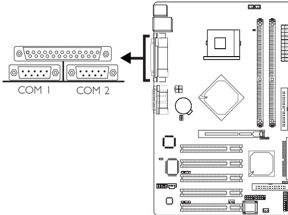
The system board is equipped with two onboard serial ports (both in Teal/Turquoise color) at locations CN6: COM 1 and CN5: COM 2.
