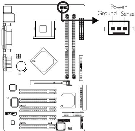
The CPU must be kept cool by using a fan with heatsink. Connect the CPU fan to the 3-pin fan connector at location J8 of the system board. The system is capable of monitoring the speed of the CPU fan.
