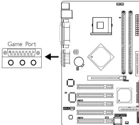
The Game/MIDI port is identical to that of a standard PC game adapter or game I/O port. Connect an analog joystick to the 15-pin D-sub connector (Gold) at location CN2 of the system board. This port works well with any application that is compatible with the standard PC joystick.
