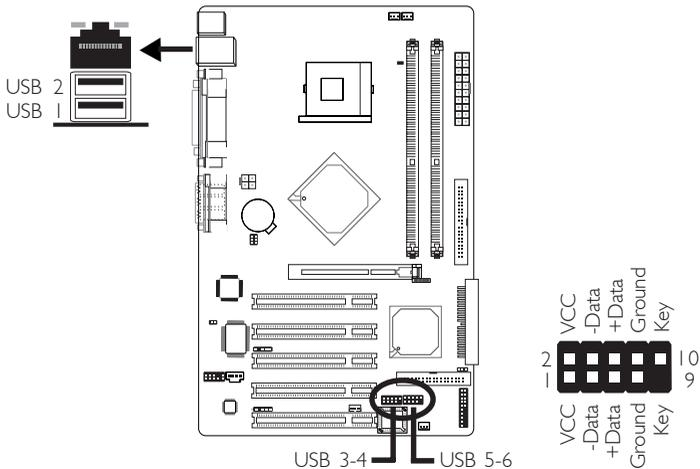
Two onboard USB 2.0/1.1 ports (Black) are at location CN7 of the system board.
