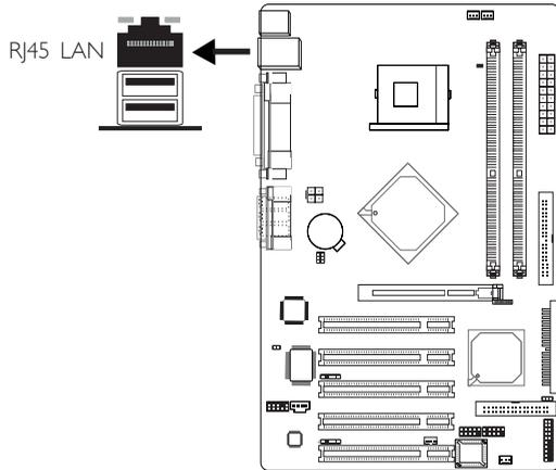
The 865PE-ALE system board is equipped with an onboard RJ45 fast-ethernet LAN port at location CN7 of the system board. It allows the system board to connect to a local area network by means of a network hub.
