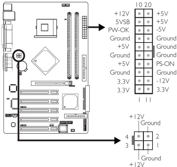
We recommend that you use a power supply that complies with the ATX12V Power Supply Design Guide Version 1.1. An ATX12V power supply has a standard 20-pin ATX main power connector and a 4-pin +12V power connector that must be inserted onto CN11 and CN10 connectors respectively.
