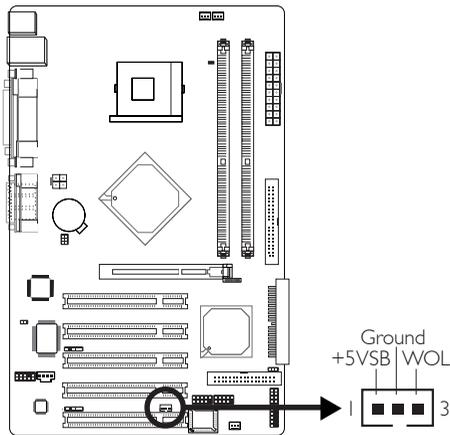
Your LAN card package should include a cable. Connect one end of the cable to the wakeup header on the card and the other end to location J6 on the system board. The network will detect Magic Packet and assert a wakeup signal to power-up the system. Refer to the add-in card's manual for details. Note: Your LAN card must support the remote wake up function.
