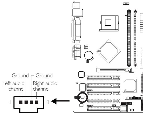
The CD-in (J3) connector is used to receive audio from a CD-ROM drive, TV tuner or MPEG card.
