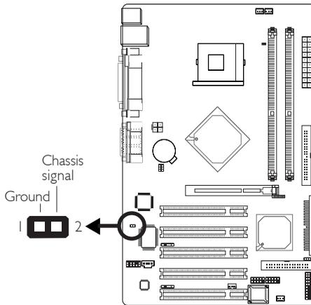
The system board supports the chassis intrusion detection function. To use this function, connect the chassis intrusion sensor cable from the chassis to J2. Whenever a chassis component has been removed, the sensor sends signal to J2 alerting you of a chassis intrusion event. To disable this function, place a jumper cap over J2.
