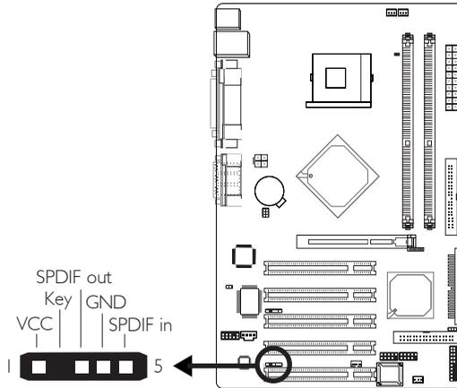
The system board is equipped with a S/PDIF connector. One card-edge bracket, mounted with S/PDIF ports, will be provided as an option. Install the card-edge bracket to the system chassis then connect the audio cable connector to J4. Make sure pin 1 of the audio cable connector is aligned with pin 1 of J4.
