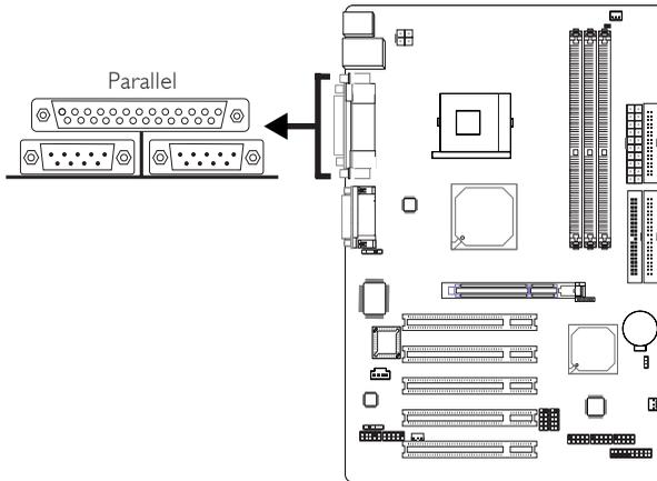
The system board has a standard parallel port (Burgundy) at location CN9 for interfacing your PC to a parallel printer. It supports SPP, ECP and EPP.
