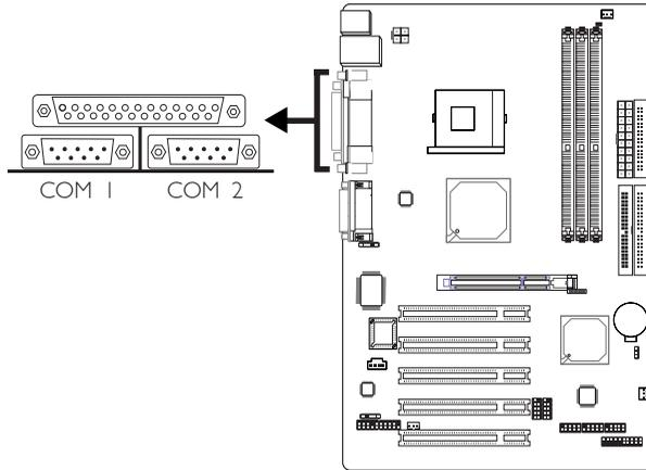
The system board is equipped with two onboard serial ports (COM 1: CN6 and COM 2: CN5) - both in Teal/Turquoise color:
