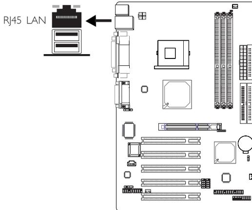
The system board is equipped with an onboard RJ45 LAN port at location CN7 of the system board. It allows the system board to connect to a local area network by means of a network hub.
