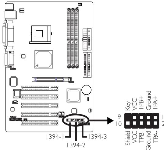
The system board is equipped with three IEEE 1394A connectors: 1394-1 (J12), 1394-2 (J13) and 1394-3 (J17). One card-edge bracket, mounted with 1394A port(s), will be provided as an option. Install the card-edge bracket to the system chassis then connect one of the cable connectors to a 1394A connector on the system board. Make sure pin 1 of the cable connector is aligned with pin 1 of the 1394A connector.
