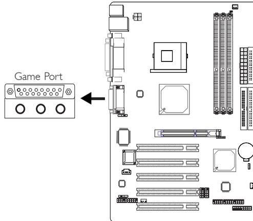
The Game/MIDI port is identical to that of a standard PC game adapter or game I/O port. Connect an analog joystick to the 15-pin D-sub connector (Gold) at location CN8 of the system board. This port works well with any application that is compatible with the standard PC joystick.
