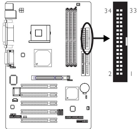
The system board is equipped with a shrouded floppy disk drive connector that supports two standard floppy disk drives. To prevent improper floppy cable installation, the shrouded floppy disk header has a keying mechanism. The 34-pin connector on the floppy cable can be placed into the header only if pin 1 of the connector is aligned with pin 1 of the header.
