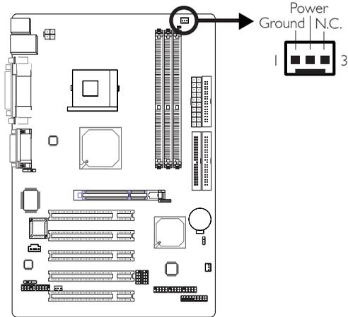
The CPU must be kept cool by using a fan with heatsink. Connect the CPU fan to the 3-pin fan connector at location J15 of the system board.
