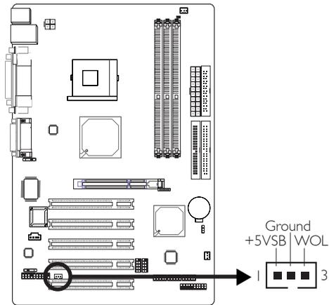
Your LAN card package should include a cable. Connect one end of the cable to the wakeup header on the card and the other end to location J8 on the system board. The network will detect Magic Packet and assert a wakeup signal to power-up the system. Refer to the add-in card's manual for details. Note: Your LAN card must support the remote wake up function.
