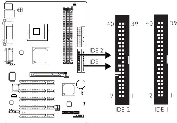
The system board is equipped with two shrouded PCI IDE headers that will interface four Enhanced IDE (Integrated Drive Electronics) disk drives. To prevent improper IDE cable installation, each shrouded PCI IDE header has a keying mechanism. The 40-pin connector on the IDE cable can be placed into the header only if pin 1 of the connector is aligned with pin 1 of the header.
