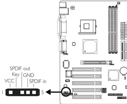
The system board is equipped with a S/PDIF connector. One card-edge bracket, mounted with S/PDIF ports, will be provided as an option. Install the card-edge bracket to the system chassis then connect the audio cable connector to J4. Make sure pin 1 of the audio cable connector is aligned with pin 1 of J4.
