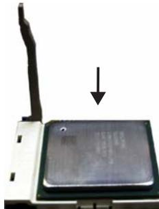
5. Once the CPU is in place, push down the lever to lock the socket. The lever should click on the side tab to indicate that the CPU is completely secured in the socket.
