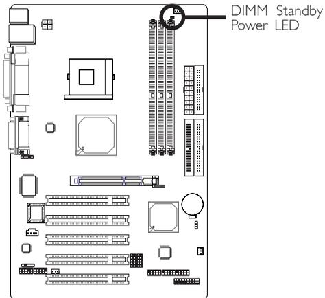
The DIMM Standby Power LED will turn red when the system's power is on or when it is in the Suspend state (Power On Suspend or Suspend to RAM). It will not light when the system is in the Soft-Off state.
