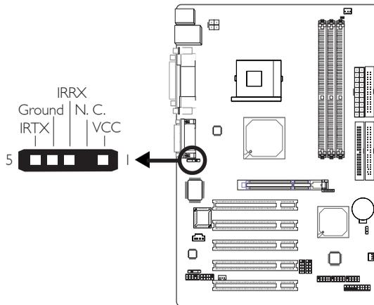
Connect your IrDA cable to connector J2 on the system board.
