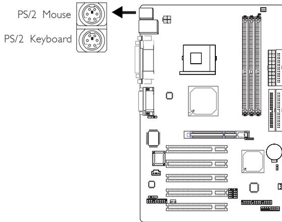
The system board is equipped with an onboard PS/2 mouse (Green) and PS/2 keyboard (Purple) ports - both at location CN1 of the system board. The PS/2 mouse port uses IRQ12. If a mouse is not connected to this port, the system will reserve IRQ12 for other expansion cards.
