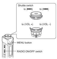
1 Set the RADIO ON/OFF switch to RADIO ON to turn on the radio.
