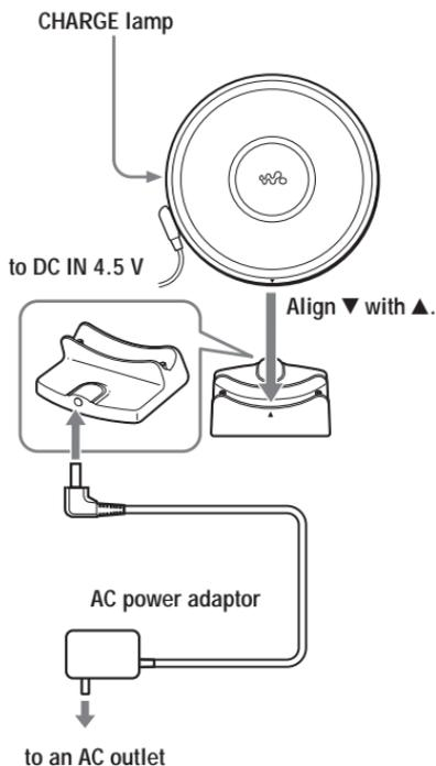
Charging of the batteries starts. In the display of the remote control, "Charging" indication flashes and the indicator sections of
