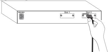
8. Power on the switch: Reconnect the previously removed power sources to the switch. Check the switch's front-panel LED indicators to ensure that the module is operating correctly. Refer to the table of LEDs on page 1 for a description of the LED indications. If the module does not respond, see "Troubleshooting" on page 7.
