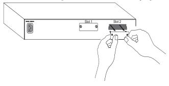
**5. Insert the new module into the switch:** Holding the new module with the text on the front panel upright, carefully slide the module into the lower slot on the rear panel, and press gently until it snaps into place. Be sure the new module's front panel is flush with the switch panel.
