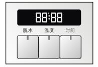
The LED display shows the data of programme which need to be setup alternately before the programme starts, such as remaining time, washing temperature, spin speed etc; only remaining time is displayed after the programme starts; displays "End" when the programme has ended; if "- - - " was selected, display" - - - " to remind there is still washing solution in the washing machine.
