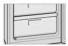
The temperature of the variable-temperature freezer compartment is adjustable between -4°C and -18°C. Under this condition, food is frozen superficially and its storage period is about two to three weeks. Food can be kept fresh for a longer time period without being frozen too hard, thus there is no need to thaw it before cooking.
