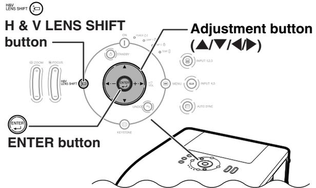
**2** Press **▲**, **▼**, **◀** or **▶** on the projector or the remote control to adjust the image position.
