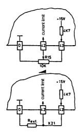
**Example 1:** Variable current limit adjustable via R15 in the range of 0-100 % I<sub>N</sub> of the internally set current limit
