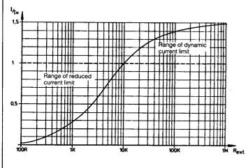
Determination of the resistance  $R_{\text{ext}}$  as a function of the desired current limit Resistance values above 10 k $\Omega$  result in a dynamic current limit > 100%  $I_{N}$
