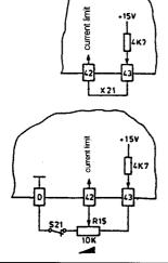
**Example 3:** Maximum current limit ( $I_{max} = 1.5 \times I_{N}$ ). The time limit is 15 s (function "Increased current limit" with LED "ESB")
