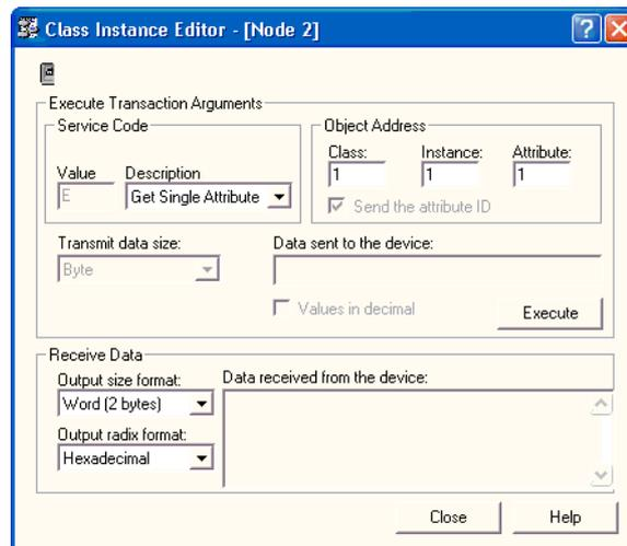
3 In the **Object Address** field, type the path of the parameter in the boxes **Class, Instance, Attribute**.
