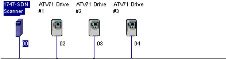
2 Right-click the DeviceNet scanner (node 00) and select **Properties**. The Scanner Module dialog box appears.
