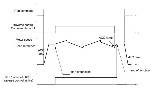
The function starts when the drive has reached its base reference and the traverse control command has been enabled. When the traverse control command is disabled, the drive returns to its base reference, following the drive ACC or dEC ramp. The function then stops, as soon as it has returned to this reference. Bit 15 of word LRS1 is at 1 while the function is active.
