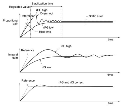
The oscillation frequency depends on the system kinematics.
