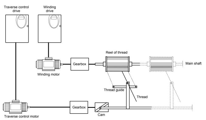
The cam speed of rotation must follow a precise profile to ensure that the reel is steady, compact and linear:
