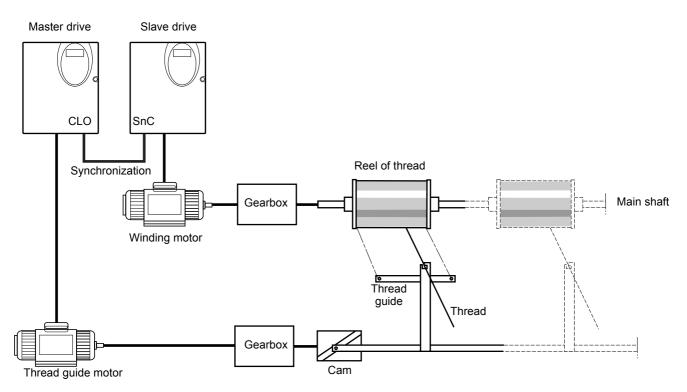
The "Counter wobble" function is used, in certain applications, to obtain a constant thread tension when the Traverse control function causes significant variations in speed on the thread guide motor (trH and trL see page <u>13</u>). **Two special "Traverse control" drives must be used (a master and a slave).**
