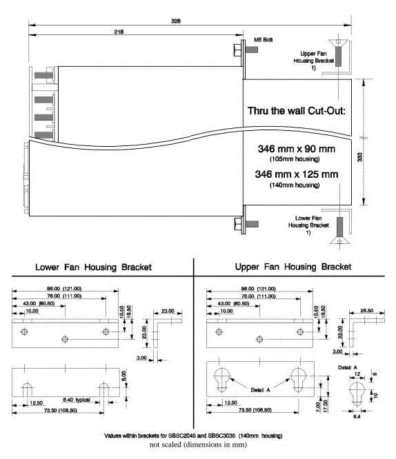
1) Upper and lower fan housing brackets are not contents of delivery. They must be ordered seperately according table below. The sets below contain both brackets and the screws.
