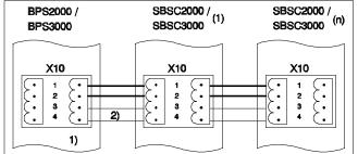
1) The shown BPS, can be replaced by an external 24V-power-supply.
