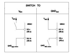
X2.x: "x" for connector pin, e.g. x=2 ? X2.9 = Enable-Input
