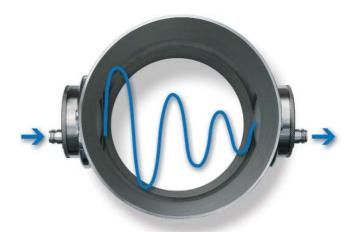
While radiating through a liquid product with microwaves they suffer a phase shift and attenuation change which directly correlates with the water content i.e. with the dry matter content of the material.
