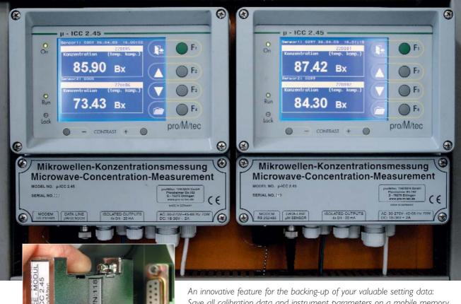
An innovative feature for the backing-up of your valuable setting data: Save all calibration data and instrument parameters on a mobile memory chip. This chip can safely remain in the controller or you can keep it in another secure place. 30 data sets can be saved. Technical modifications reserved!
