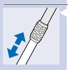
Adjust the tube to the length you find most comfortable during vacuum cleaning.
