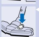
Push the rocker switch on top of the nozzle with your foot to make the brush strip come out of the housing. At the same time the wheel will be lifted to prevent scratching and to increase manoeuvrability.
