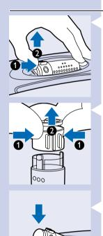
Place your thumb and index finger on the sides of the cartridge. Remove the cartridge from the holder by pressing on the disc
