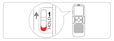
2 Slide the HOLD switch down to the Off position to disengage the keypad lock.
