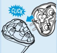
► If the shaving unit becomes detached from the shaver, check whether the hinge spring is still properly attached, i.e. has not come loose and does not show any cracks or damage. If the hinge spring is still properly attached, the shaving unit can be easily put back on the shaver again. However, if the hinge spring has come loose, is cracked or damaged, please contact your Philips dealer or the nearest Philips service centre to avoid damage to your shaver.
