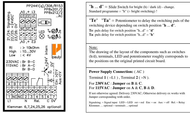
Depending on the construction, the output of the hole detector's switching device is at the relay contact ( = terminal 3, 4, 5; floating contact) or in the case of an electronics output with p-n-p transistor switching to 24V DC / "0" V ( = terminal 6; terminal 7 = ground).
