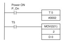
TIM5 is started when the power is turned ON. After 0.1 to 0.2 s (100 to 200 ms) elapses, the TIM5 contact turns ON and the analog input 1 conversion data stored in word 2 is transferred to DM0.
