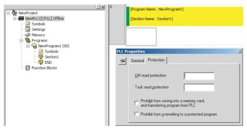
3. Connect online and select **PLC - Transfer - To PLC** to transfer the program. The tasks registered in step 2 will be password-protected.
