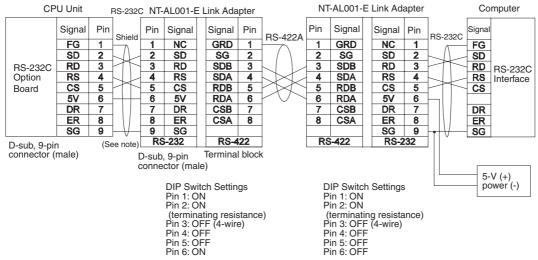
**Note** We recommend using the following NT-AL001-E Link Adapter Connecting Cables to connect to NT-AL001-E Link Adapters.
