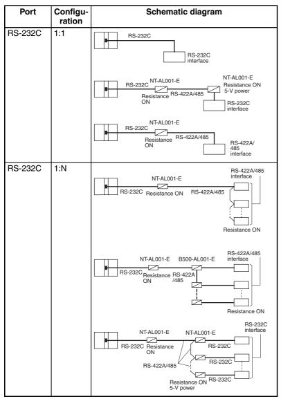
**Note** (1) The maximum cable length for RS-232C is 15 m. The RS-232C standard, however, does not cover baud rates above 19.2 Kbps. Refer to the manual for the device being connected to confirm support.
