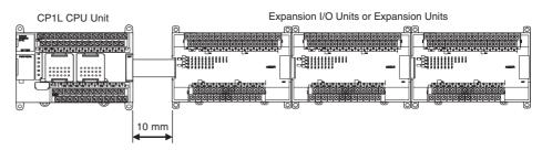
If sufficient space cannot be provided between the CPU Unit and the first Expansion Unit or Expansion I/O Unit, use the PLC in an ambient temperature of 0 to 50°C.
