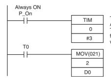
TIM 0 will start as soon as power turns ON. After 0.2 to 0.3 s (200 to 300 ms), the input for TIM 0 will turn ON, and the converted data from analog input 0 that is stored in word 2 will be transferred to D00000.
