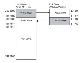
CP1L is set as the link master, so CIO 3000 to CIO 3007 are its write area. Any data written to these words with the OUT or MOV instructions will be automatically transferred to LR 00 to LR 07 in the CPM2A. The CPM2A will use these words as its read area.
