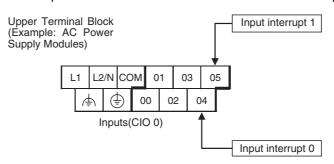
Input Terminal Block of CPU Units with 14 I/O Points
