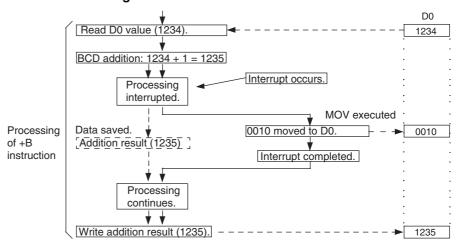
The interrupt occurs during processing of the +B instruction and the result is saved temporarily without being written to the destination word (D0).
