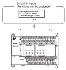
**Note** Settings in the PLC Setup determine whether each input point is to be used as a normal input, interrupt input, quick-response input, or high-speed counter.
