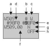
11. Press the **OK** button to enter the Change Screen of I/O memory W509. The following table shows the setting items.
