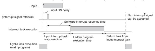
The time from completing the ladder program in the input interrupt task until returning to cyclic task execution is 60 µs.
