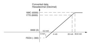
Current in the 4 to 20 mA range corresponds to hexadecimal values 0000 to 1770 (0 to 6,000). The range of data that can be converted is FED4 to 189C hex (-300 to 6,300). Current in the range of 3.2 to 4 mA is expressed as two's complement.
