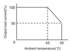
(3) CP1W-32ER's maximum number of simultaneously ON output points is 24 (75%). Design the system considering the simultaneously ON points and load current based on the following curve.
