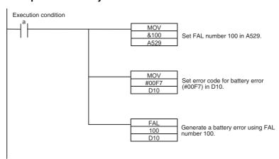
**Note** Use the same methods as for actual system errors to clear the simulated system errors. Refer to the *10-2 Troubleshooting* for details. All system errors simulated with FAL(006) and FALS(007) can be cleared by cycling the power supply.
