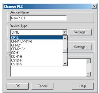
2. Click the **Settings** Button by the *Device Type* Field and, when the Device Type Settings Dialog Box is displayed, set the *CPU Type* Field to *J*, *L*, *L10* or *M*.
