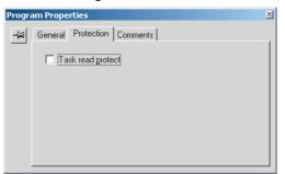
2. Display the *Protection* Tab of the PLC Properties Dialog Box and register a password in the *Task read protection* Box.
