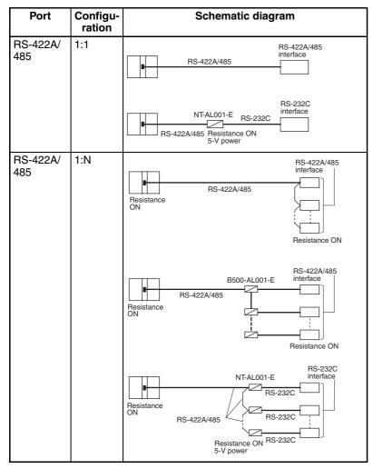
**Note** (1) The maximum cable length for RS-232C is 15 m. The RS-232C standard, however, does not cover baud rates above 19.2 Kbps. Refer to the manual for the device being connected to confirm support.
