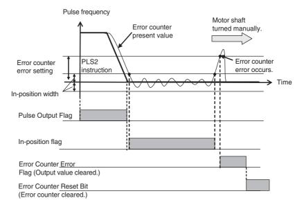
Low-speed Operation Using Minimum Output Setting An inductive motor driven with an inverter is different from a servomotor in that the torque at low speeds is so low that it may not be possible to turn the motor shaft at the minimum frequency. The CP1L provide a minimum output setting the ensure a minimum output to enable positioning at low speeds even when there are extremely few pulses in the error counter.
