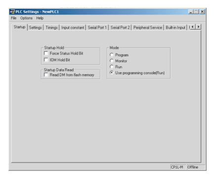
**Note** A Programming Console cannot be connected to a CP1L CPU Unit. If *Use programming console* is set, the CPU Unit will start in RUN mode.
