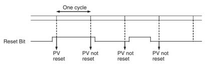
**Note** The comparison operation can be set to stop or continue when a high-speed counter is reset. This enables applications where the comparison operation can be restarted from a counter PV of 0 when the counter is reset.
