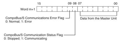
Write the data to be transmitted to the Master Unit in the output word (n+1).
