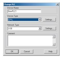
2. Click the **OK** Button to finish setting the PLC model. Then connect to the CP1L by executing the CX-Programmer's online connection command.
