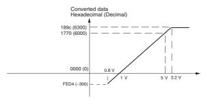
Voltage in the 1 to 5 V range corresponds to hexadecimal values 0000 to 1770 (0 to 6,000). The range of data that can be converted is FED4 to 189C hex (-300 to 6,300). Voltage in the range of 0.8 to 1 V is expressed as two's complement.
