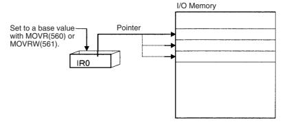
**Note** It is possible to specify regions outside of I/O memory and generate an Illegal Access Error when indirectly addressing memory with Index Registers. Refer to *Appendix E Memory Map* for details on the limits of PLC memory addresses.
