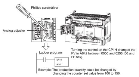
Changing Settings Using External Analog Setting Inputs External analog values of 0 to 10 V (resolution: 256) are converted to digital values and stored in a word in the AR Area. This enables applications that require on-site adjustment of settings that do not demand a particularly high degree of accuracy, such as for example, a setting based on changes in outdoor temperatures or potentiometer inputs.
