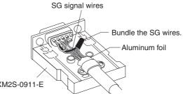
**Note** The Hood (FG) is internally connected to the ground terminal (GR) on the CPU Unit. Therefore, FG is grounded by grounding the ground terminal (GR) on the power supply terminal block. Although there is conductivity between the Hood (FG) and pin 1 (FG), connect the Hood (FG) to the shield because the Hood (FG) has smaller contact resistance with the shield than pin 1 (FG), and thus provides better noise resistance.
