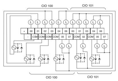
AC-power-supply models have a 24-VDC output terminals (+/-) on the lower terminal block. They can be used as a DC power supply for the input circuit.
