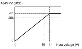
The maximum input voltage is 11 VDC. Do not apply a voltage greater than that.
