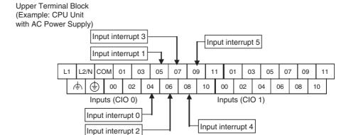
Input Terminal Block of CPU Units with 60 I/O Points
