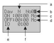
Press the **OK** button to enter the Day Timer Screen. The final digit of the Timer No. will be flashing. The following table shows the setting items.
