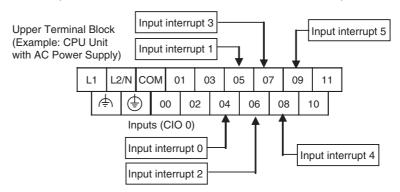
Input Terminal Block of CPU Units with 30 I/O Points
