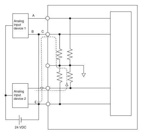
Example: If analog input device 2 is outputting 5 V and the same power supply is being used for both devices as shown above, approximately 1/3, or 1.6 V, will be applied to the input for input device 1.
