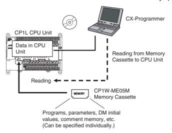
This function can be used for operations such as writing the required backup data to the CPU Unit for maintenance.
