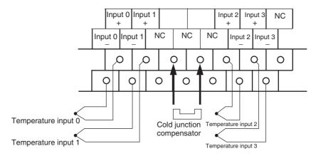
**Note** When using a Temperature Sensor Unit with a thermocouple input, observe the following precautions:
