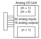
"m" is the last allocated input word and "n" the last allocated output word on the CPU Unit or previous Expansion Unit or Expansion I/O Unit.
