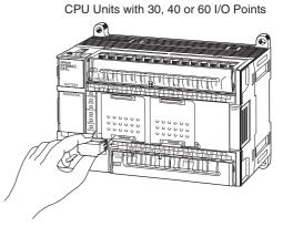
2. Holding the Memory Cassette with the side with the nameplate facing upwards, insert the Memory Cassette all the way into the slot.
