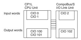
The input word (m+1) contains the 8 bits of data from the Master Unit and two CompoBus/S communications flags.
