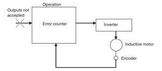
Referencing the Automatically Calculated Inverter Frequency Command Value If the following settings are made in the PLC Setup, the inverter frequency command value will be calculated automatically and set in A23 in the Auxiliary Area. These settings are on the Inverter Positioning 0 Tab Page in the PLC Setup.
