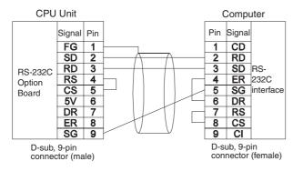
Using NT-AL001-E Converting Link Adapters
