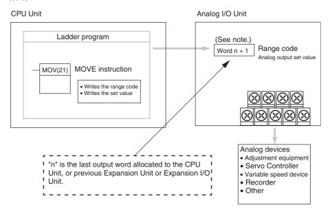
**Note** Word (n + 1) can be used for either the range code or the analog output set value.
