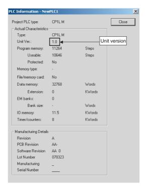
Use the above display to confirm the unit version of the CPU Unit.
