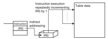
The Index operation uses the following procedure.
