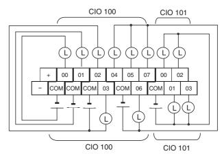
AC-power-supply models have a 24-VDC output terminals (+/-) on the lower terminal block. They can be used as a DC power supply for the input circuit.
