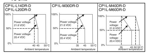
**Note** The above restrictions, apply to the relay output load current from the CPU Unit even if Expansion I/O Units are not connected.
