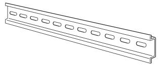
Secure the DIN Track to the control panel using M4 screws separated by 210 mm (6 holes). The tightening torque is 1.2 N·m.
