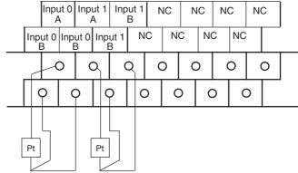
Temperature input 0 Temperature input 1
