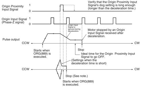
Note: The Origin Input Signal can be detected immediately after the Origin Proximity Input Signal goes from ON to OFF if the deceleration time is short, e.g., starting from within the Origin Proximity Input Signal.
