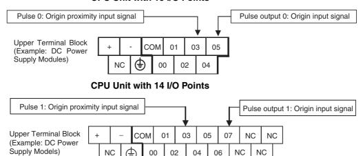
Pulse output 0: Origin input signal
