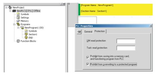
3. Either select *PLC - Transfer - To PLC* to transfer the program or select *PLC - Protection - Set Password* and click the **OK** button.
