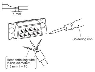
4. Return the heat-shrinking tube to the soldered portion, then heat the tube to shrink it in place.
