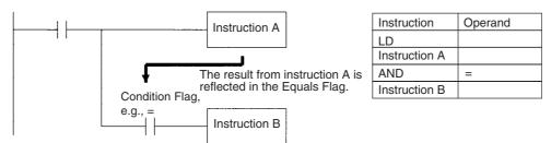
Since the Condition Flags are shared by all of the instructions, program operation can be changed from its expected course by interruption of a single task. Be sure to consider the effects of interrupts when writing the program. Refer to SECTION 2 Programming of CS/CJ Series Programming Manual (W394) for more details.
