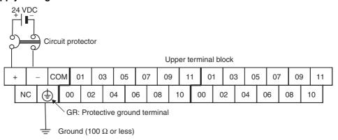
• Use crimp terminals or solid wire for wiring the power supply. Do not connect bare stranded wires directly to terminals.
