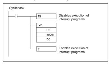
b. The following example shows duplicate processing by an interrupt task, which interrupts processing while BSET is writing to a block of words and yields an incorrect comparison result.
