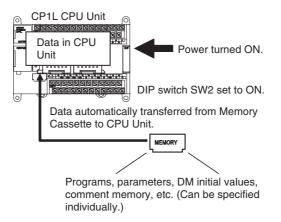
This function can be used to copy data to another CPU Unit without using the CX-Programmer.
