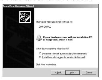
3. The following window will be displayed. Click the Browse Button for the Include this location in the search Field, specify C:\Program Files\OMRON\CX-Server\USB\win2000\_XP\Inf, and then click the Next Button. The driver will be installed. ("C:\" indicates the installation drive and may be different on your computer.)
