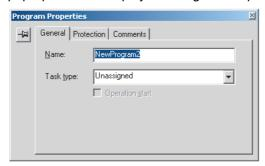
3. Set the *Task type* in the Program Properties Window. In this example, interrupt task 140 was allocated to NewProgram2.
