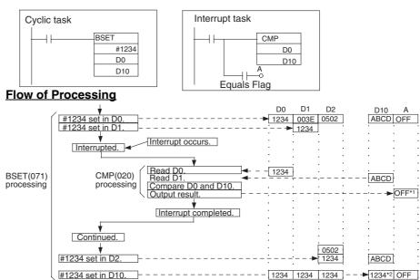
Since the interrupt occurs during BSET(071) processing and before #1234 is set in D10, the content of D0 and D10 do not match when the comparison is made in the interrupt task (\*1) and output A remains OFF.
