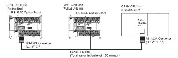
Note The CP1W-CIF11 is not insulated, so the total transmission distance for the whole transmission path is 50 m max. If the total transmission distance is greater than 50 m, use the RS-422A/485 port on the CP1W-CIF12 directly, or the insulated NT-AL001-E, and do not use the CP1W-CIF11. If the CP1W-CIF12 or NT-AL001-E is used, the total transmission distance for the whole transmission path is 500 m max.
