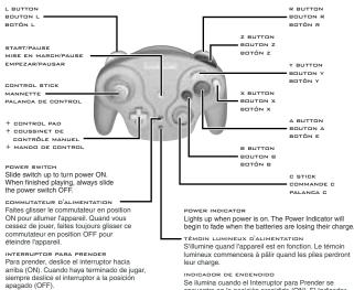
Lights up when power is on. The Power Indicator will begin to fade when the batteries are losing their charge.
