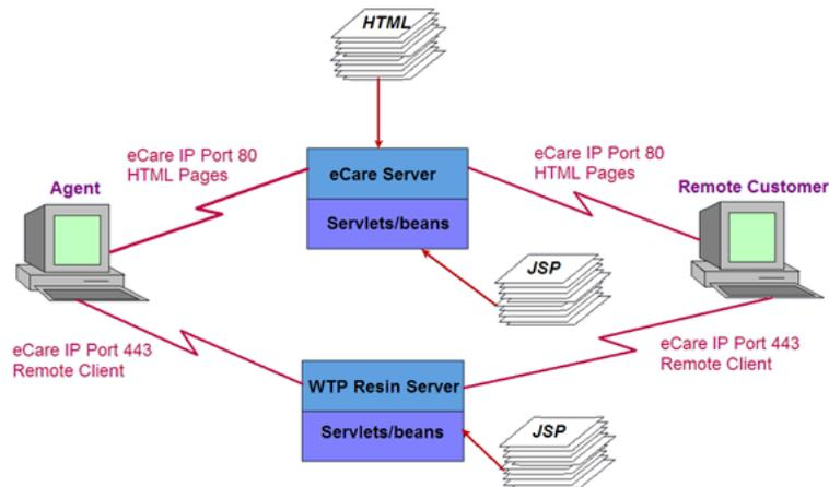
**eCare Page Server** A Resin server that handles requests associated with eCare HTML and JSP pages. The eCare page server has an Internet-available IP address and runs on port 80.
