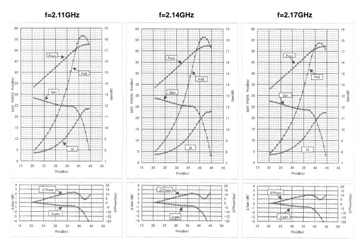
Test Condition: Vds=12V,Idq=4A,Ta=25deg.C
