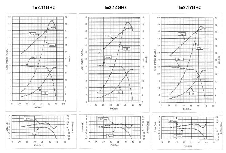
Test Condition: Vds=12V,Idq=2A,Ta=25deg.C
