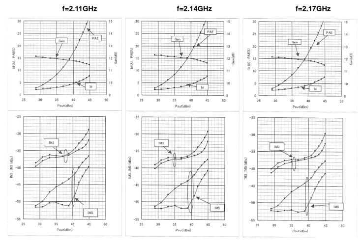
Test Condition: Vds=12V,Idq=2A,Ta=25deg.C
