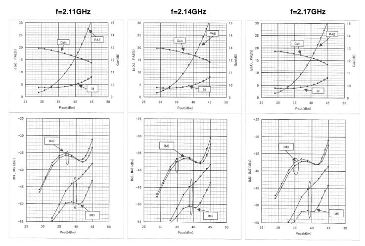
Test Condition: Vds=12V,Idq=4A,Ta=25deg.C
