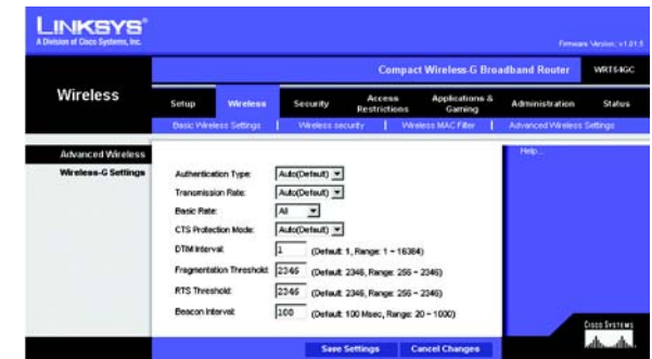
Figure 5-21: Wireless Tab - Advanced Wireless Settings
