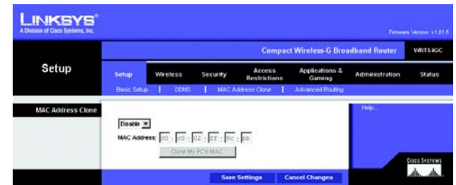
Figure 5-11: Setup Tab - MAC Address Clone
