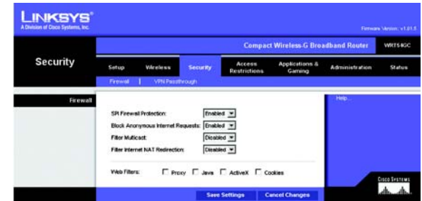
Figure 5-22: Security Tab - Firewall
