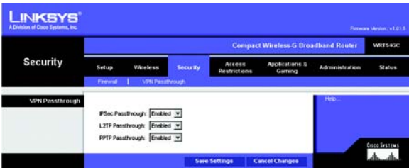
Figure 5-23: Security Tab - VPN Passthrough
