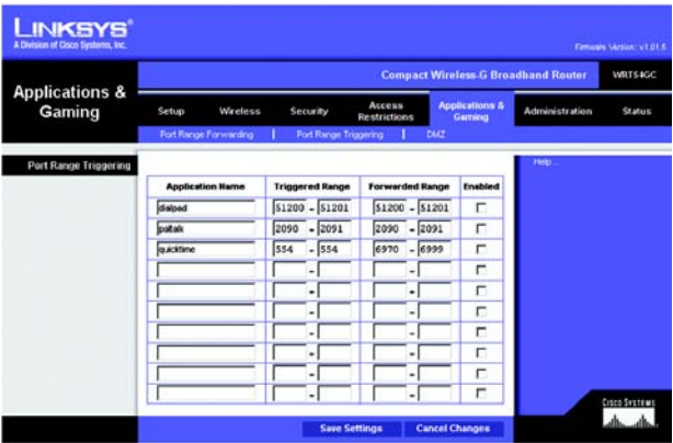
Figure 5-28: Applications and Gaming Tab - Port Triggering
