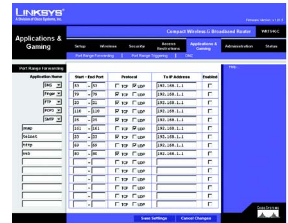
Figure 5-27: Applications and Gaming Tab - Port Range Forwarding
