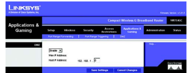
Figure 5-29: Applications and Gaming Tab - DMZ
