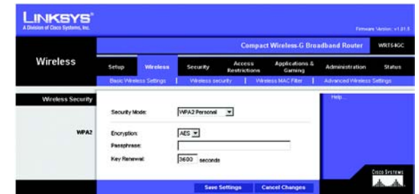
Figure 5-17: Wireless Tab - Wireless Security (WPA2 Personal)
