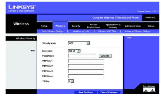
Figure 5-15: Wireless Tab - Wireless Security (WEP)
