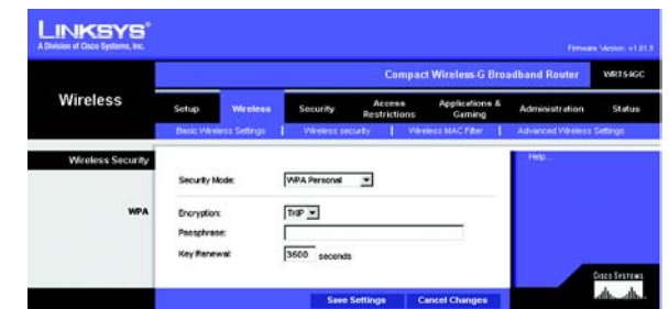
Figure 5-16: Wireless Tab - Wireless Security (WPA Personal)
