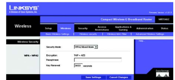
Figure 5-18: Wireless Tab - Wireless Security (WPA2 Mixed Mode)
