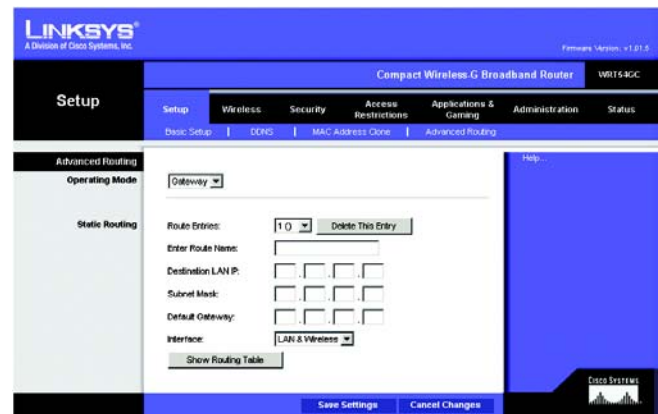
Figure 5-13: Setup Tab - Advanced Routing (Router)
