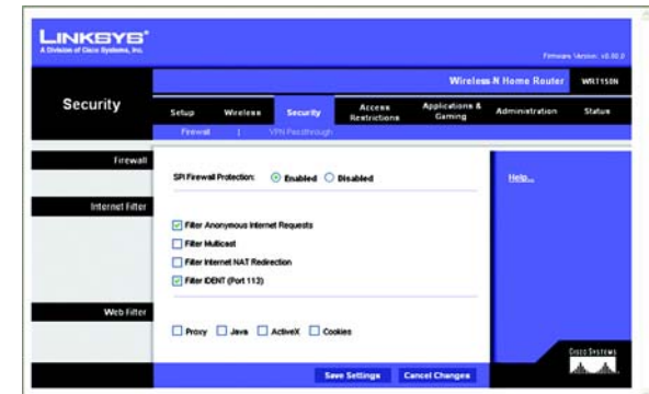
Figure 5-24: Security Tab - Firewall
