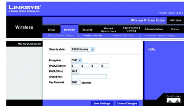
Figure 5-17: Wireless Security - PSK-Enterprise
