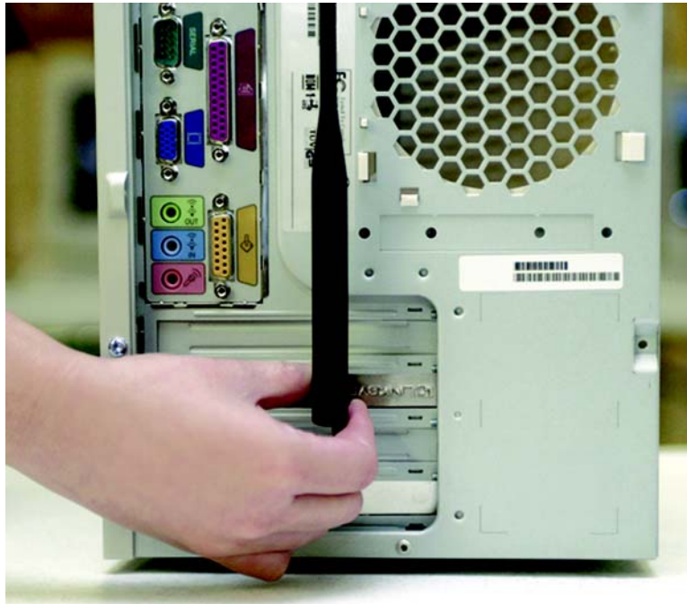
Figure 4-2: Proper Positioning of the Antenna
