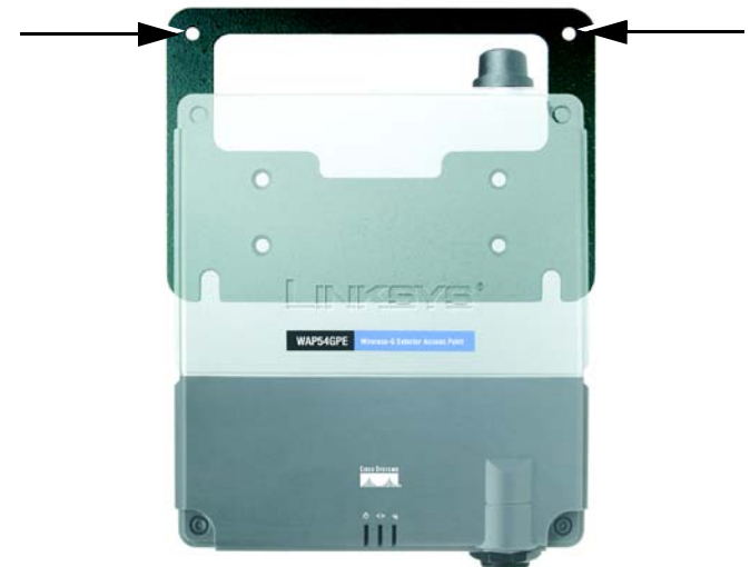
Figure 4-3: Ground the Access Point
