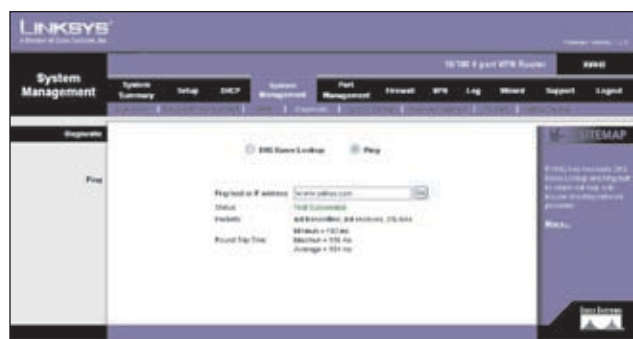
System Management &gt; Diagnostic &gt; Ping
