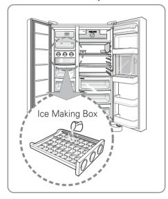
■ Ice will be dropped into the ice storage bin by rotating ice separation handle of ice making compartment.
