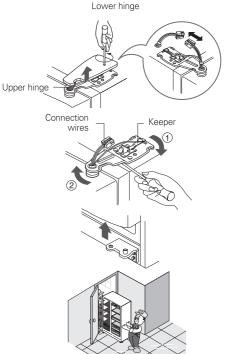
If the height of freezer compartment door is different from the height of Refrigerator compartment door
