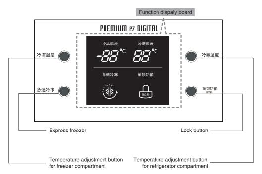
How to adjust the temperature in the freezer compartment
