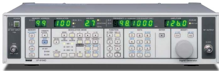
The model VP-8194D signal generator with FM stereo modulator and RDS + ARI generator. Built-in CENELEC compliant RDS / ARI signal source and RDS 16-pattern memory. Included editor software (Windows) allows RDS data to be easily downloaded through RS-232-C interface and edited on a PC.
