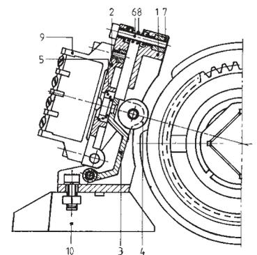
Fig. 1.1.4: Switching Element Actuator GSW100
