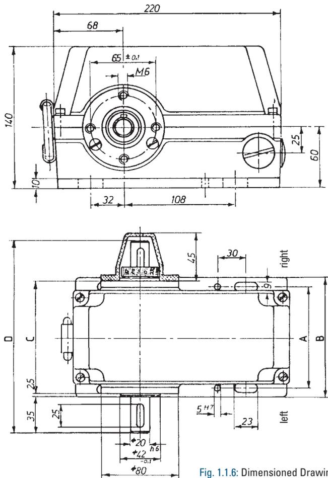
Fig. 1.1.6: Dimensioned Drawing GSW100
