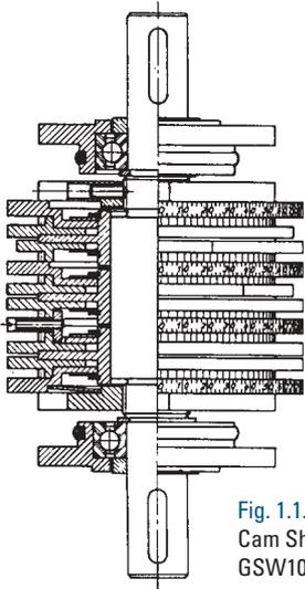
Fig. 1.1.5: Cam Shaft GSW100-03
