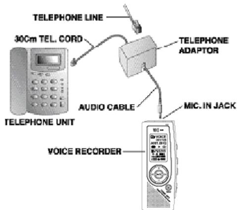
CONNECT LINE - IN CABLE TO THE MICROPHONE JACK ON THE VOICE RECORDER AND TELEPHONE ADAPTOR. CONNECT TELEPHONE CABLE TO TELEPHONE ADAPTOR. PRESS "REC" BUTTON FOR RECORDING. IF YOU SET UP THE "ARS", AUTOMATICALLY START RECORDING IF THERE IS ANY SOUND AND PAUSING IF THERE IS NO SOUND.
