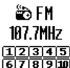
FOR THE AUTOMATIC TUNING, PRESS AND HOLD FORWARD OR REWIND BUTTON FOR 2 SECONDS. THE TUNER AUTOMATICALLY SCANS AND STOPS ON THE NEXT STATION WITH A STRONG SIGNAL. IN AN AREA WITH WEAK RECEPTION, PRESS THE FAST FORWARD OR REWIND BUTTON TO FIND A CLEAR STATION.
