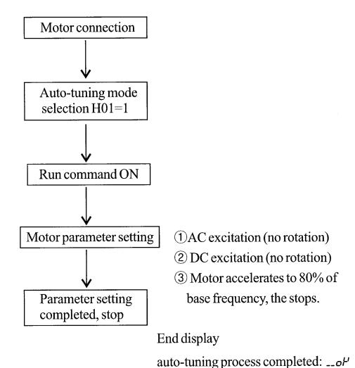
**Note)** The motor parameter of N50 is standard data of HYUNDAI standard 4-poles motor. At the sensorless vector control when using different poles motor, operates by using auto-tuning data as a motor parameter.
