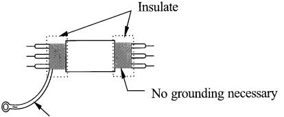
Connect to the common terminal[CM1] and [L] of the inverter
