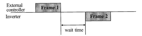
Frame start: Frame start is recognized by signal line data transmitted.
