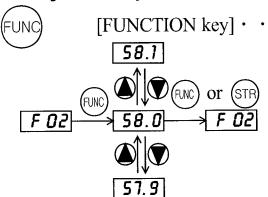
[FUNCTION key] · · This key allows the selection of commands and memorises parameters. When the key is pressed once in the state of, the extension function code selection state is set.
