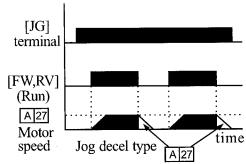
0:Free-run stop 1:Deceleration stop 2:DC braking stop
