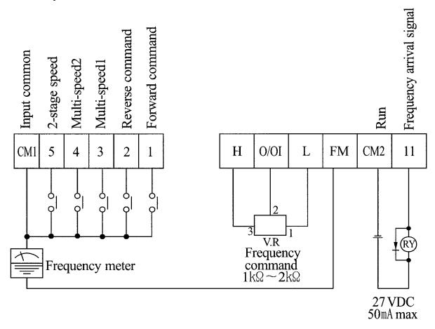
**Note1)** When an output intelligent terminal is used, be sure to install a surge absorbing diode in parallel with relay. Otherwise, the surge voltage created when the relay goes ON or OFF may damage the output intelligent terminal circuit.
