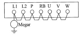
Never test the withstand voltage on the inverter. The inverter has a surge protector between the main circuit terminals and the chassis ground.
