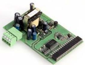
A green PCB with a transformer and other power-related components, designed for providing a 24V supply.                                                                                                              |
