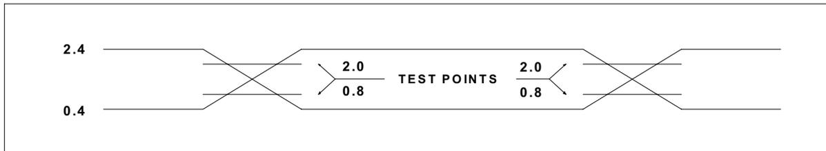
AC Testing : Input is driven at 2.4V for logic "1",and 0.4V for logic "0".Timing measurements are made at 2.0V for logic "1",and 0.8V for logic "0".
