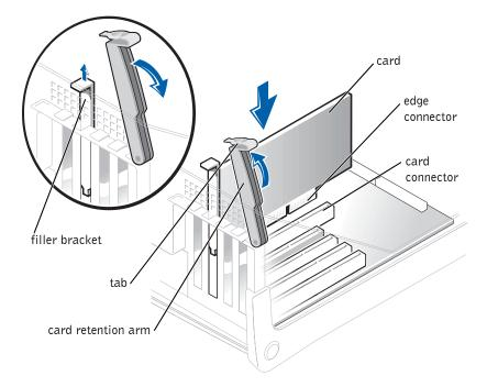
6 Press the tab on the card retention arm and raise the retention arm.
