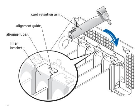
**NOTICE:** Do not route card cables over or behind the cards. Cables routed over the cards can prevent the computer cover from closing properly or cause damage to the equipment.
