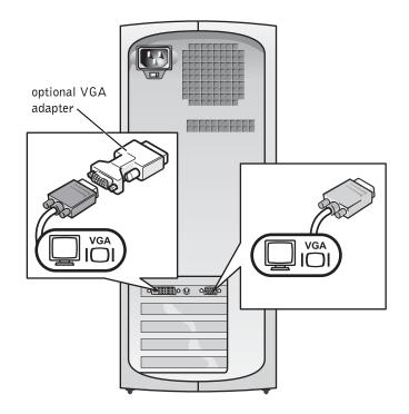
If one monitor has a VGA connector and the other one has a DVI connector:
