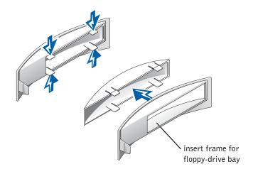
6 Reattach the empty insert frame over the front of the drive bay. The insert frame fits only one way.
