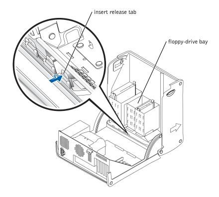
**4** From outside the computer, pull the insert away from the computer's front panel.
