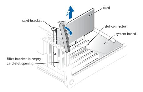
7 If you are removing the card permanently, install a filler bracket in the empty card-slot opening.
