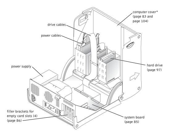
\*Depending on the types of drives installed in your computer, the cover may not open as widely as shown in the figure.
