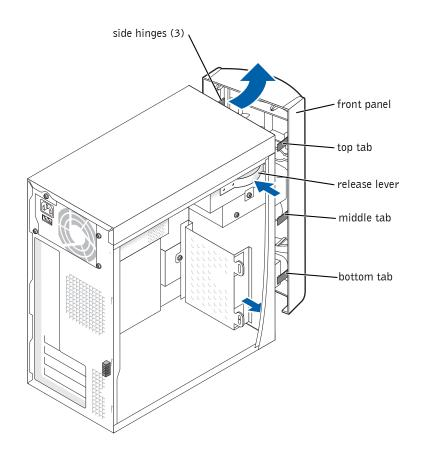
**7** Press in the two insert tabs, and then push out the front-panel insert.
