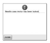
Touch **CLOSE** to automatically reset the needle bar case.
