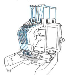
Not all six needles can be used to sew at the same time. Only one needle is moved to the embroidering position at a time. According to the sewing order, the needle bar case is moved to the left and right so that the needle bar and needle thread with the required color can be moved to the embroidering position.
