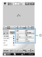
(1) The threads threaded on the needle bars are indicated as shown here.
