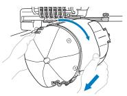
• Be careful that the cap frame does not hit any nearby parts, such as the presser foot. After removing the brim holder, unlock the snap lock of the clamping frame, remove the clips, and then remove the cap.
