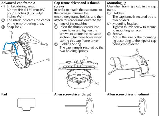
• Use when adjusting the ring of the cap frame driver and the height of the L-shaped bracket. (Refer to page 229.)
