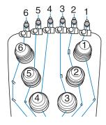
Pass the thread through the number 1 hole in the thread guide just above the spool, and then pass the thread through the number 1 hole in the thread guide toward the front of the machine.
