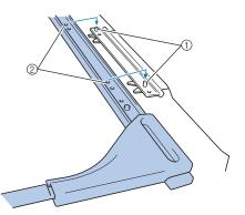
① Pins in the frame-mounting plate
