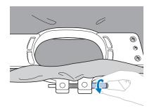
If the screw was tightened using a discshaped screwdriver, use the included discshaped screwdriver to loosen it.
