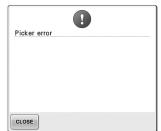
A saved combined pattern is being The thread picker did not operate The thread trimming button was correctly. Remove the thread entangled on the thread picker.
