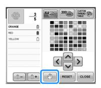
The mark appears to indicate where the machine will stop.
