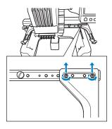
Remove the right arm, align the pins on the embroidery frame holder with the holes in the arm, as shown in the illustration, and then insert the screws removed in step and tighten them.
