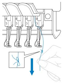
Continue pulling the thread until the knot is above the needle. Cut the knot.
