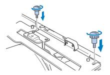
While pushing in the cap frame driver toward the machine so that it is fully inserted, tighten the two lower thumb screws to secure the cap frame driver.
