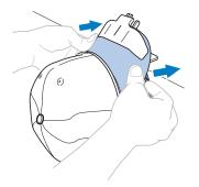
This completes the positioning of the cap in the cap frame.
