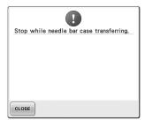
The machine was stopped while the needle bar case was moving.
