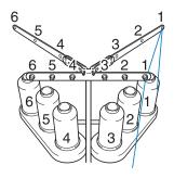
Place on spool pin 1 the spool of thread with the color (lime green) specified for needle bar 1.
