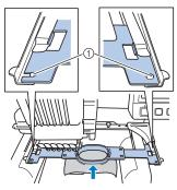
Make sure that the pins on the left and right arms of the embroidery frame holder fit into the positioning slot and hole on the embroidery frame.
