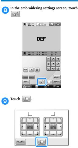
The needle bar is positioned in the lowerleft corner of the pattern. The embroidery frame moves so that the needle is positioned correctly.
