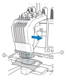
Needle at the embroidering position The needle is positioned over the hole in the needle plate (2).
