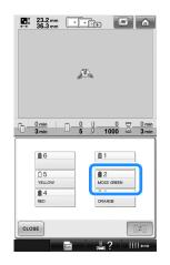
**3** Touch the number of the other needle bar that will be switched. The two needle numbers are connected with an arrow.
