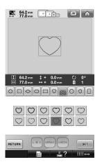
Select a frame pattern sewn with straight stitches to embroider onto the fabric for the appliqué. Carefully cut outside of the stitching.
