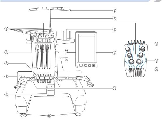
① Thread tension knobs
