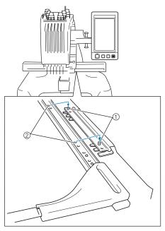
Pins on the frame-mounting plate
