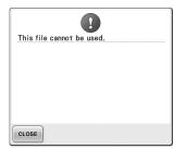
The file format is incompatible with this machine. Check the list of compatible file formats. (Refer to page 202.)
