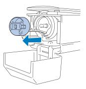
3 Rotate the handwheel (about 50 degrees) to move the race of the hook to a position where it can easily be oiled.
