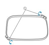
Loosen the screw on the outer frame.
