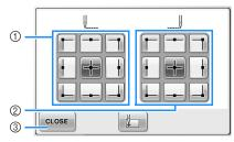
① Specifies the starting position Specifies the ending position 2 Touch a key to select the setting. The highlighted key shows the currently selected setting.
