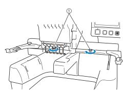
Use the thumb screws included with the machine (thumb screws removed in step 1 on page 227).
