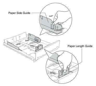
For Legal size paper, press and hold the universal guide release button as you slide out the front of the paper tray.
