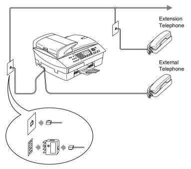
When you are using an external or extension telephone, the LCD shows Telephone.
