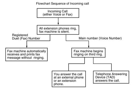
After you have set the FaxAbility feature to On, the receive mode is set to Manual automatically. Unless you have a TAD or Voice Mail set up on the FaxAbility number, Manual mode means you must answer all the call yourself. You can not change the receive mode to the other mode while the FaxAbility is set to on.
