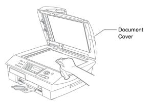
Clean the white bar and the glass strip under the film with isopropyl alcohol on a lint-free cloth.
