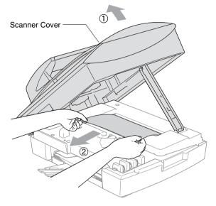
If the paper is jammed underneath the print head, disconnect the MFC from the power source so you can move the print head and take out the paper. **3** If you can not pull out the jammed paper, remove the Jam Clear Cover. Pull the jammed paper out of the MFC.
