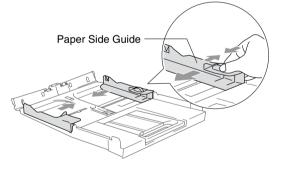
**3** Pull out the paper support and unfold the paper support flap.
