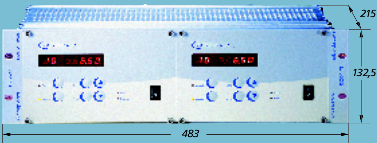
19" rack with 2 channels approx. 5.5 kg
