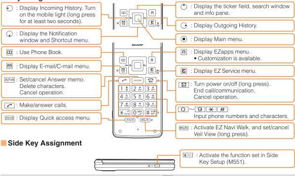
• If you lose track of where you are or if you make a mistake, press 2070/15 to return to the previous screen. Return to the standby screen by holding down 😭 for at least one second.
