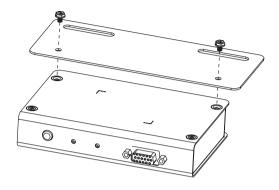
3. Screw the bracket into any convenient location on the rack.
